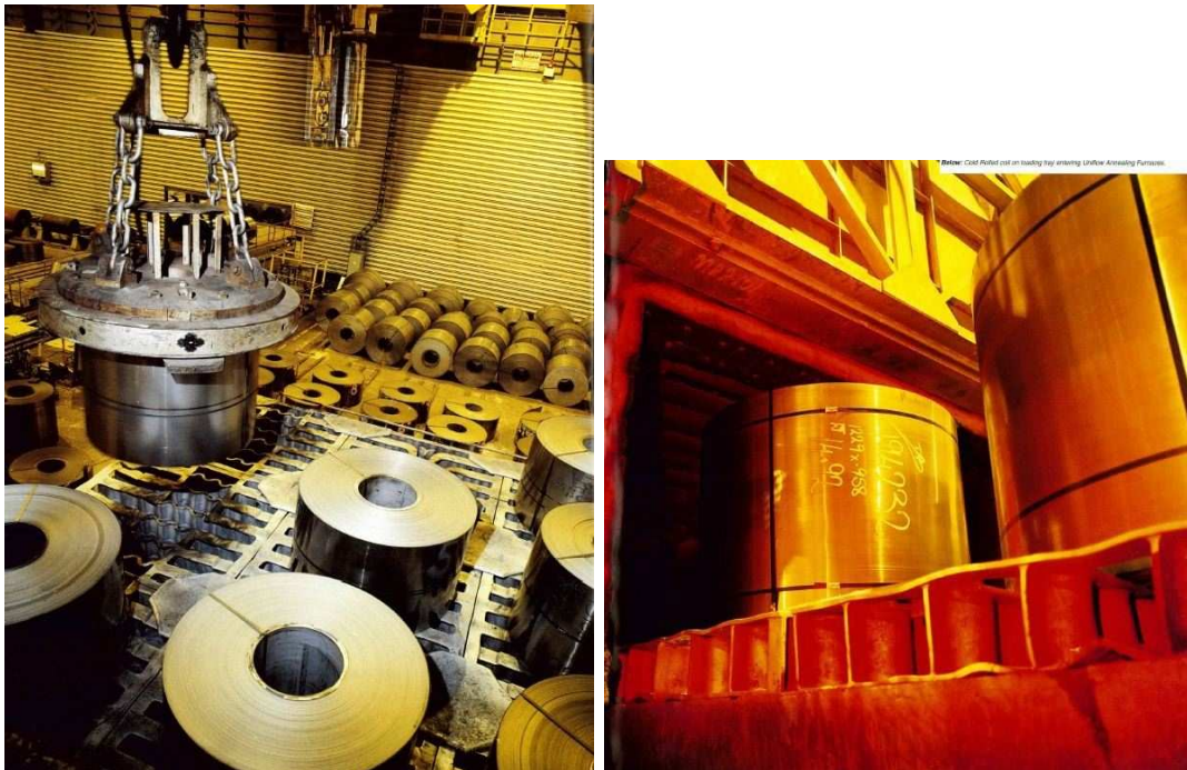
Figure 1: Photographs of steel coils being prepared for and entering the UAS furnace. (Photographs courtesy of NZ Steel.)
